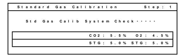
**3.** If the system is normal, the following display will appear. Select OK and press the ENTER Key to start calibrating the  $CO_2$  and  $O_2$  density. After calibration, return to normal cultivating operation.
